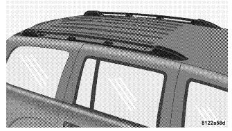
The load carried on the roof when equipped with a luggage rack must not exceed 68 kg (150 lbs.), and should be uniformly distributed over the cargo area.
